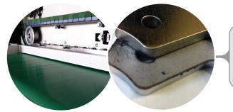
The cross belts aggressively round inside and outside contours to while lightly touching the surface. Consumables per part are significantly lower than media used in hand tools. Manual labor is reduced up to 10:1. This presents unbeatable economics with ROI's less than one year even for low volumes in many cases.
